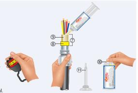
8. Re-insert the barrier pot sub-assembly 🗇 back into the inner ②.
